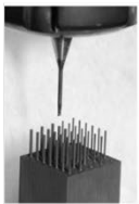
Micro milling of Graphite electrodes
